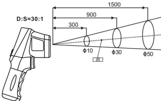
3. Field of view: Make sure the target is larger than the unit's spot size. The smaller the target the close measure distance. When accuracy is critical, make sure the target is at least twice as large as the spot size.
