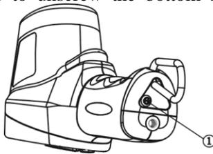
2. Catch the hook and pull the cover of battery out from the bottom;
