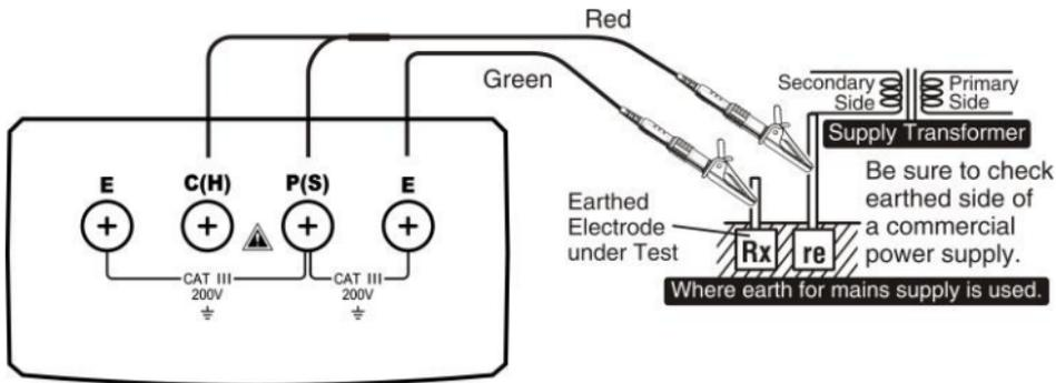
Risk: Be careful of electric shock when using commercial electric system earth method for test.
