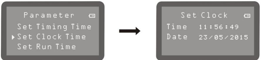
you can modify Flashing digital of the Time or date via pressing UP (or DOWN) buttons. And Press ENTER to the cursor turn to the next number.
