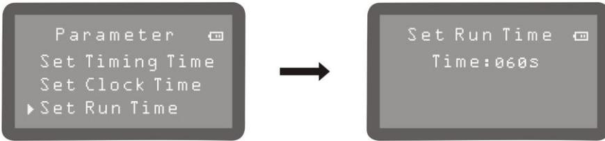
Running time is a measurement of PM2.5 time. The range of values can be set to 000, or 060 seconds -180 seconds timing measurements, if set to 000 seconds (000 seconds at the timing when the non-state) manually start or stop the measurement.
