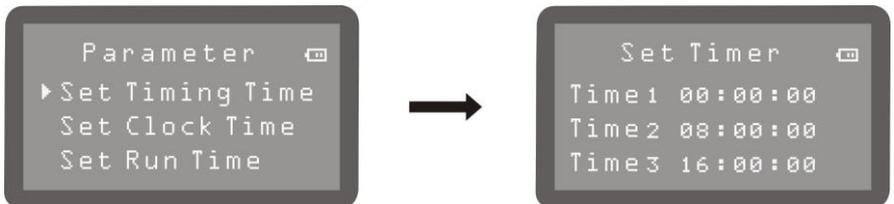
In this interface it can be setting the hour and minute about Time 1, Time 2, Time 3. you can modify Flashing digital of the Time or date via pressing UP (or DOWN) buttons. And Press ENTER to the cursor turn to the next number.
