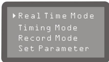
Press “UP” Key or “DOWN” Key to select “Real Time Mode” or “Timing Mode” or “Record Mode” or “Set Parameter” and Press “ENTER” Key to enter the corresponding mode.
