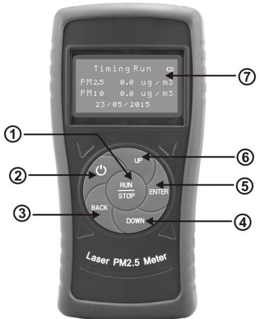
① RUN/STOP Key: Press the key to run the measurement or stop the measurement at Real Time Mode.
